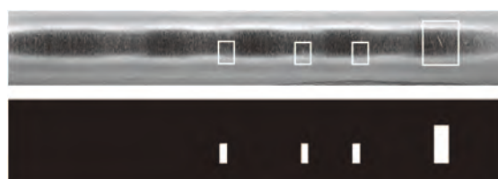
Fig. 7 Examples of microphotograph (upper row) and detection result (lower row) of dent marks
