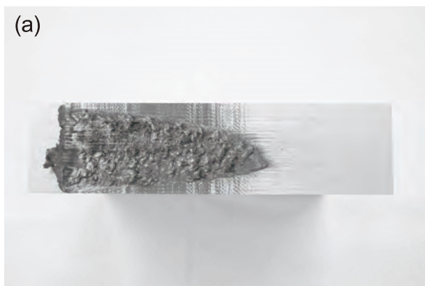
Fig. 3 Machined surface of titanium alloy prepared by milling process using (a) nonimproved, and (b) improved tools
