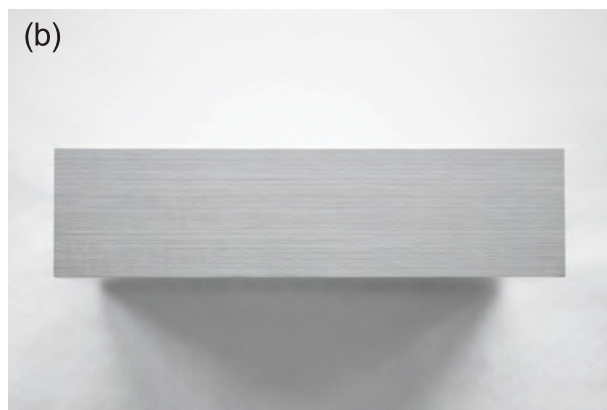
Fig. 3 Machined surface of titanium alloy prepared by milling process using (a) nonimproved, and (b) improved tools
