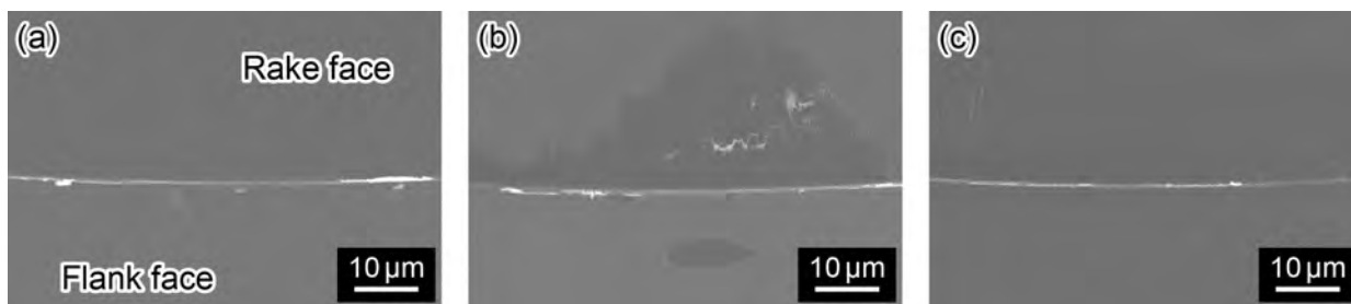
Fig. 2 SEM image of the diamond tool after machining aluminum alloy. (a) nonirradiated tool, (b) FIB irradiated tool and (c) FIB irradiated tool with heat treatment.
