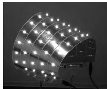
Fig. 3 Optical image of flexible sheet for LED.
