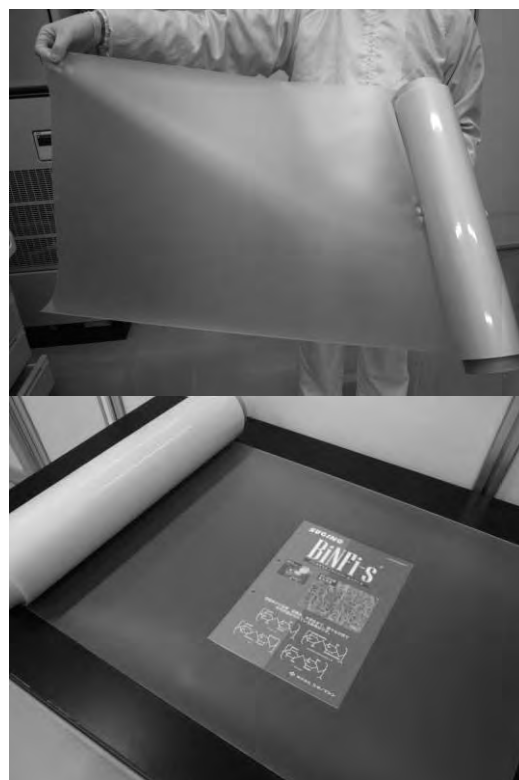
Fig.1 The trial manufacture product of the large film made of the cellulose nanofiber, BiNFi-s.
