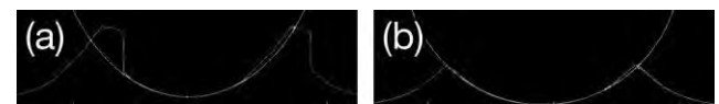
Fig. 3 Cross-sectional image of the machined surface under (a) conventional and (b) improved conditions, after machining 100000 holes.
