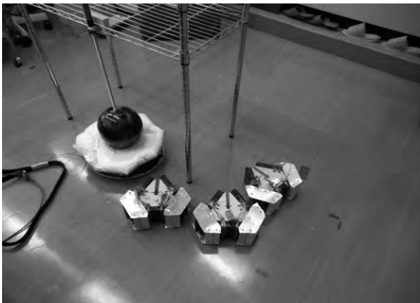
Fig. 1 Equipment pressurizing on cushion and measuring its deformation for estimates of softness or degrees of liquefaction by vibration
