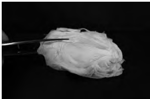
Fig. 2 A spongy aggregate of electrospun silk nanofibers.
