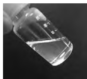
Fig. 4 The acetylated gel could collapse by ultrasonic treatment and diffuse into a nonpolar solvent, chloroform.
