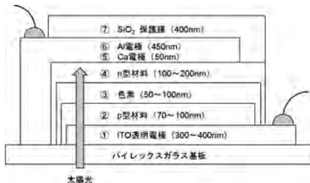
Fig. 1 Structure of organic thin-film solar cell.
