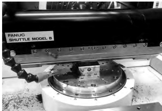
Fig. 1 Experimental setup for machining nickel phosphorus layer using ultra-precision cutting machine with shuttle unit
