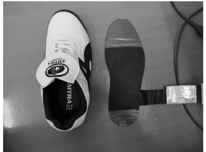
Fig. 1 Shoe and the pressure sensor
