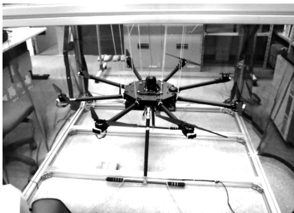
Fig. 1 Multi-copter for upper inspection with 8 rotor arms
