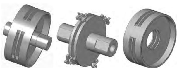
(a) Whole model (b) Shaft part (c) Outer ring part Fig. 1 Friction damping wheel model with opposing disc-shaped comb structure
