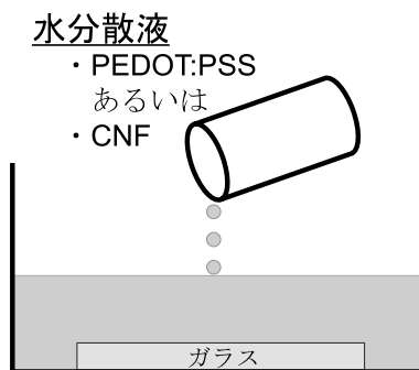
Fig. 1 Schematic diagram of casting method
