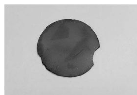
Fig. 2 Pressure sintered cathode substrate
