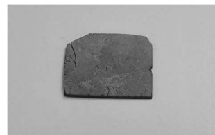
Fig. 3 Cathode substrate layered solid electrolyte
