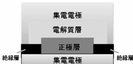
Fig. 1 Multilayer film structure
