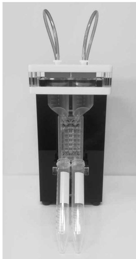
Fig. 1 Picture of the size-sorting device with the size-sorting cartridge and 15mL collection tubes
