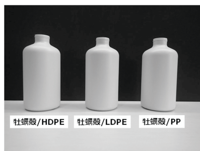
Fig. 1 Prototype of plastic bottles mixed oyster shell
